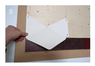
Select the main tile required for the position above the bottom left tile. Using the mounting pegs, place this tile into position on the mounting boards and insert the two left pegs only, leaving the holes on the right of this tile open.
